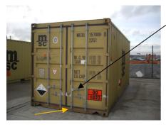
Container seals have to be fitted at the right container door – the inner locking bar /handle- only. Or as shown right
